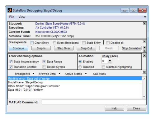
Simulation pauses after 350 seconds because of an out-of-range data error:
