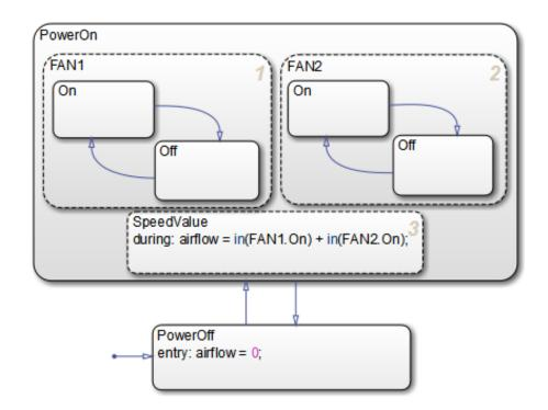
**5** Repeat the same procedure to add default transitions at the top edges of FAN1.0ff and FAN2.0ff.
