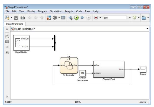
When you define one or more input events for a chart, Stateflow software adds a single trigger port to the block. External Simulink blocks can trigger the input events via a signal or vector of signals connected to the trigger port.
