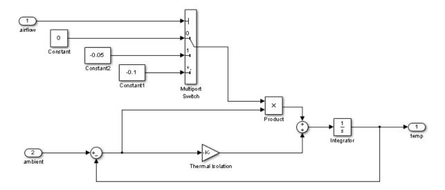
In this model, the internal temperature of the plant attempts to rise to achieve steady state with the ambient air temperature, set at a constant 160 degrees (as shown in "How the Stateflow Chart Works with the Simulink Model" on page 2-6). The rate at which the internal temperature rises depends in part on the degree of thermal isolation in the plant and the amount of cooling activity.
