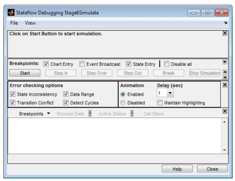
The **Browse Data** option appears grayed out, but becomes active when simulation pauses at a breakpoint. You will use this option in "Simulating the Air Controller Chart" on page 8-9.
