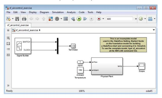
The model is incomplete because it does not include the Stateflow chart that you will build as you work through the exercises in this guide. Instead, the model contains several nonfunctional blocks: the Terminator, Inport, and Annotation blocks.
