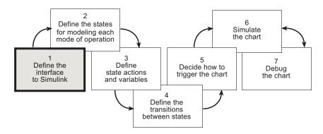
In phase 1 of this workflow, you define the interface to the Simulink model.
