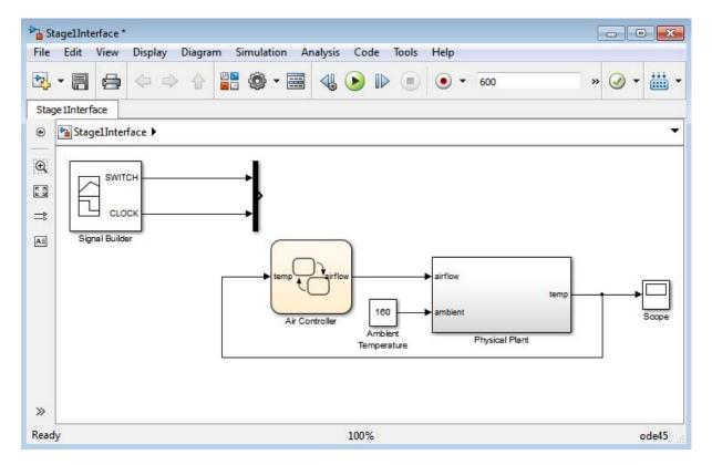
**Tip** To reposition connections, move your cursor over the end of the line. When the cursor changes to a circle, select the end of the line with the left mouse button and drag the line to a new location. For more information, see "Connect Blocks".
