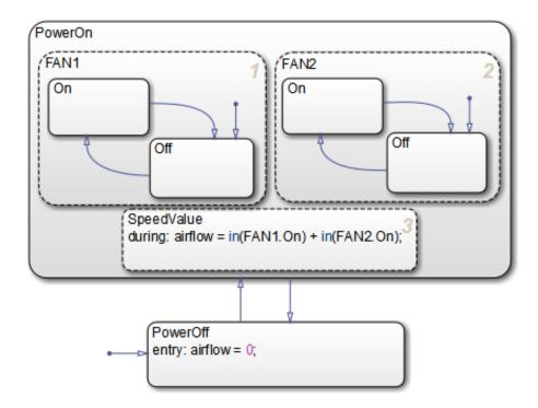
**Tip** The location of the tail of a default transition determines the state it activates. Therefore, make sure that your default transition fits completely inside the parent of the state that it activates. In the Air Controller chart pictured above, notice that the default transition for FAN1.0ff correctly resides inside the parent state, FAN1. Now consider this chart:
